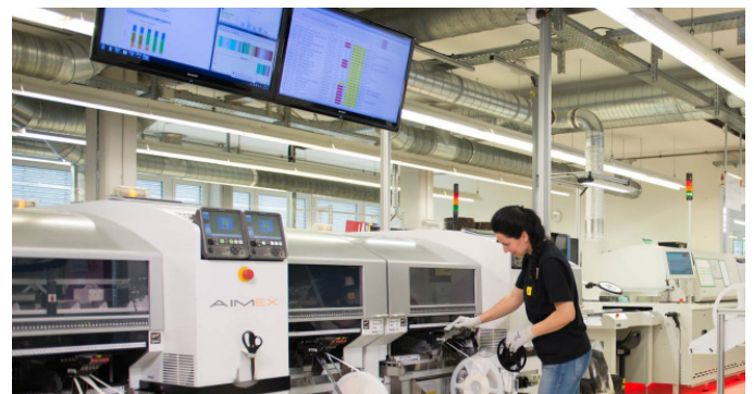
SMT Assembly – Assembly of up to 100 components per single board a lateral precision accuracy < 40 micrometers
