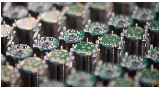
Precision milling – milling of singulated boards with a xy mechanical precision below 50 micrometers
