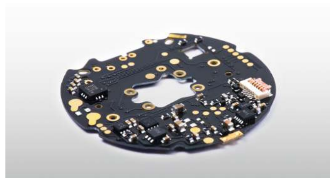
Smartwatch board – high precise electronic board for use in a smartwatch or wearable device
